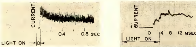
Fig. 3—Oscilloscope traces of triggered current in CdSe powder.
