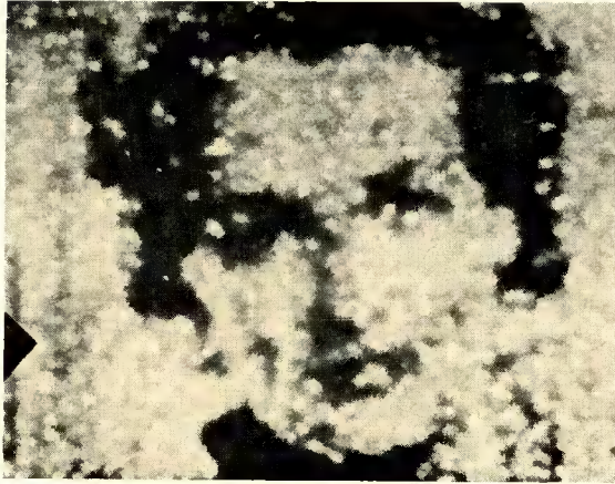
Fig. 6—Output image on 3-inch panel produced by short exposure to half-tone input image.
